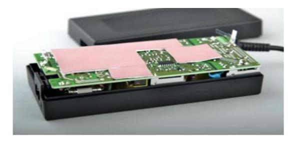
Thermal gap pad with silicon cloth to prevent needle piercing
