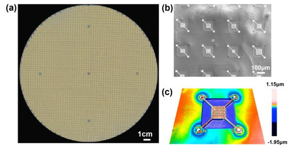
Figure 4: (a) The optical image of sensor device arrays on an 8-inch wafer; (b) SEM image of the device array; (c) 3D confocal image of the device unit.
