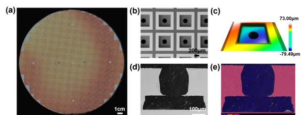
Figure 5: (a) The optical image of silicon cap arrays on an 8-inch wafer; (b) SEM image of the cap array; (c) 3D confocal image of the cap unit; (d) Cross-sectional SEM image of a bonded cap unit; (e) EDS mapping of the bonded cap unit.
