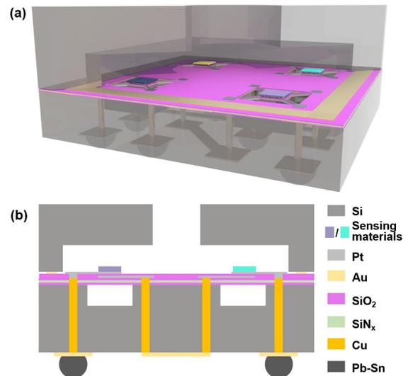
Figure 1: The schematic structure of the wafer level packaging and TSV based multimode sensor chip: (a) 3D structure; (b) 2-dimensional cross-sectional structure.
