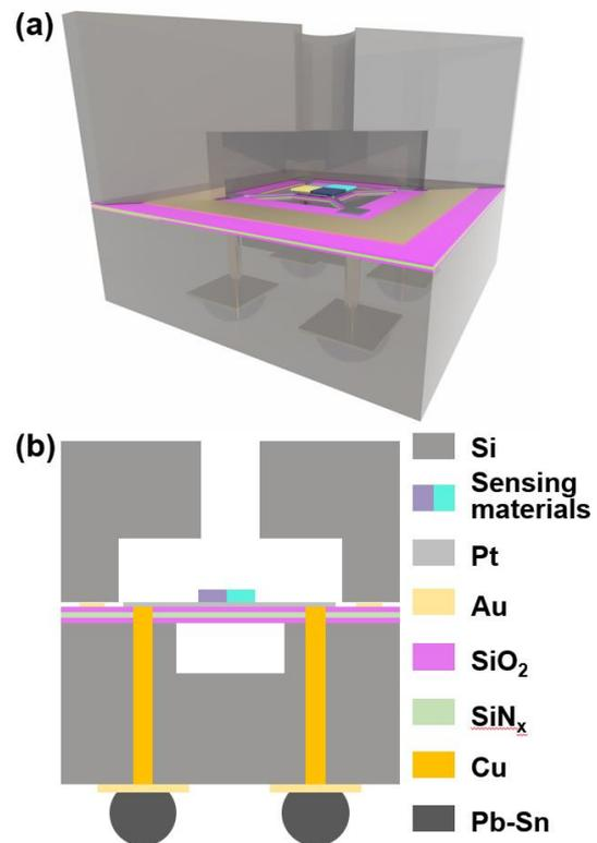
Figure 2: The schematic structure of the pattern recognition based multimode sensor chip: (a) 3D structure; (b) 2-dimensional cross-sectional structure.
