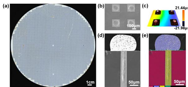
Figure 3: (a) The optical image of TSV connected solder ball arrays on an 8-inch wafer; (b) SEM image of the solder ball array; (c) 3D confocal image of the solder ball
