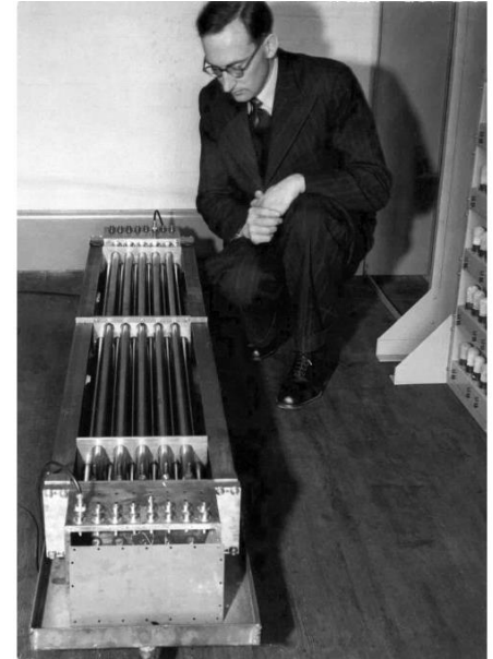
EDSAC mercury delay lines. M.V. Wilkes pictured. Courtesy of the Computer Lab at Cambridge University
